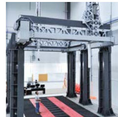
Large Gantry Inspection Unit
